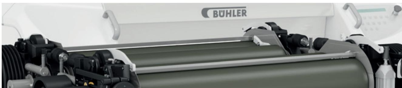
Sensor strip for roller temperature monitoring .
