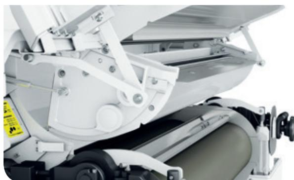
Patented feeder module with pivoting function.
