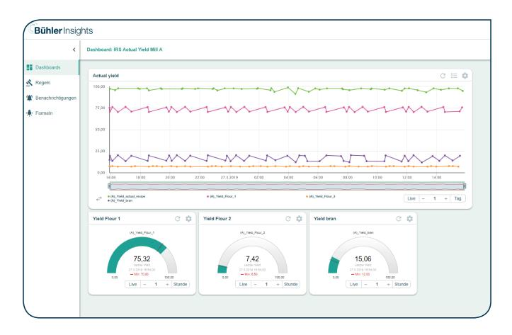
Bühler's YMS integrates data from defined scales directly into Bühler Insights, independent of the plant control system. Visualize and compare various lines against one each other. Thanks to the online data collection even those of plants in different locations. Keep track of recipe based yields over time to improve your overall mill performance.
