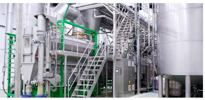
The value of the rearing residue can be increased by a pelletizing and sanitation process
