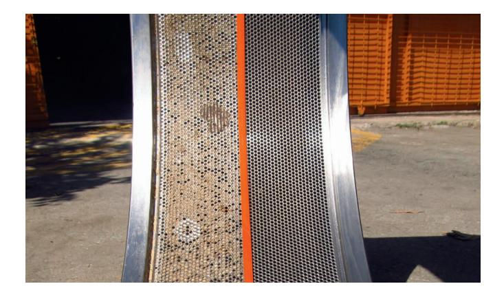
As the service life of pelleting dies proceeds, their performance declines. Plugged or shut holes, irregular wear or damaged die sections degrade the pellet quality and reduce production capacity. Selective die service extends the lifetime of your dies and cuts your operational costs.
