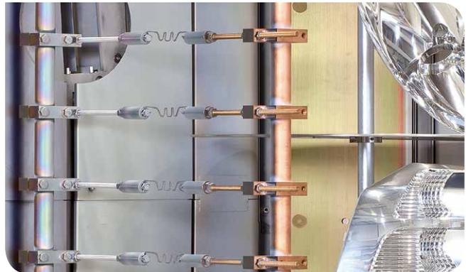
Spring filament holder inside process chamber
