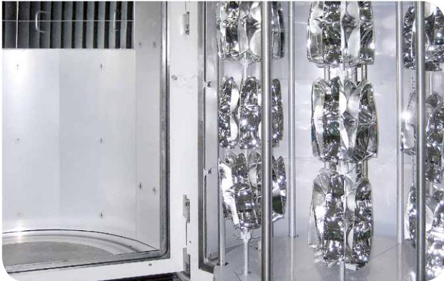
Door fully loaded with substrates
