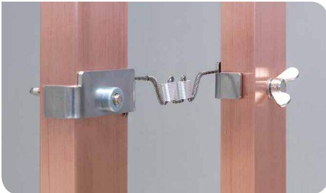
Screw filaments loaded with Al coils
