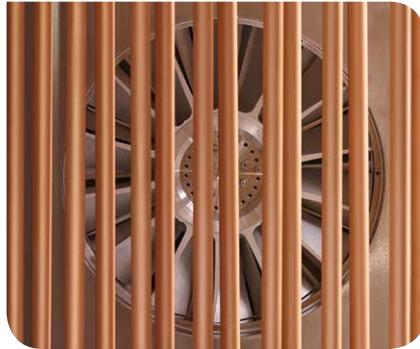
Turbomolecular pump behind cold trap
