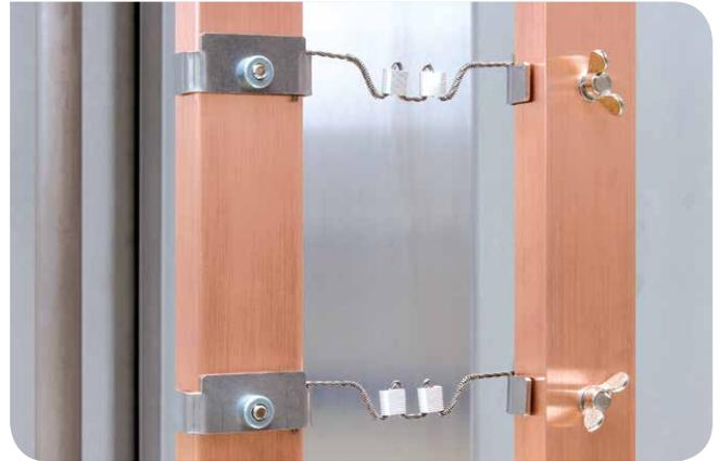
Evaporator and substrate inside the chamber
