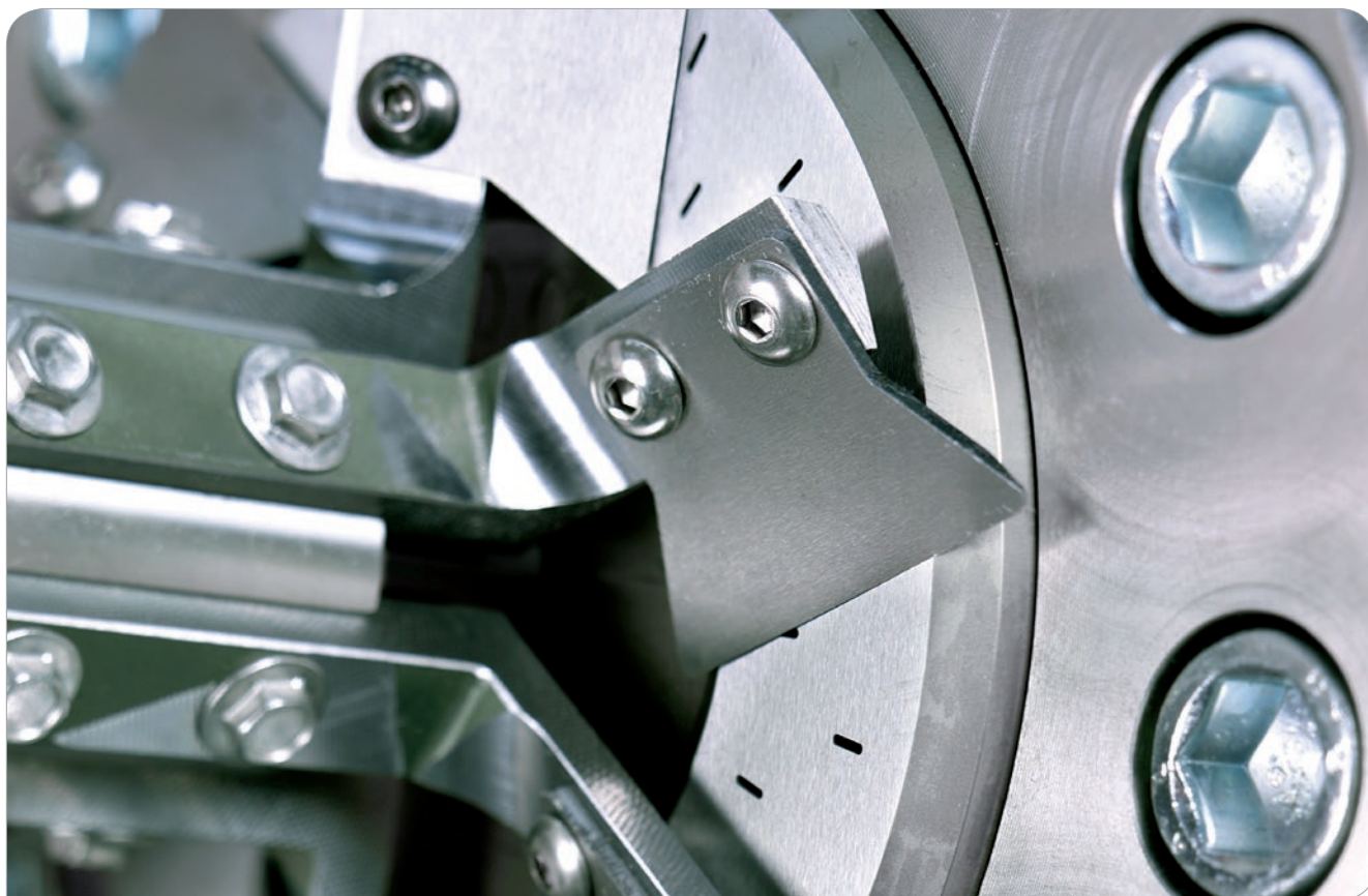
The cutting apparatus moves laterally to allow exchange of the knife head even during production.
