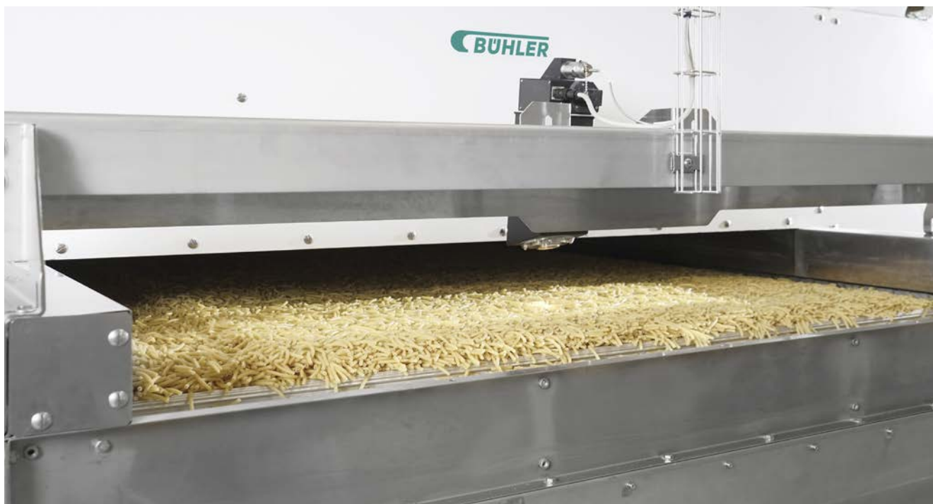
Sensor measuring moisture of short-goods pasta.
