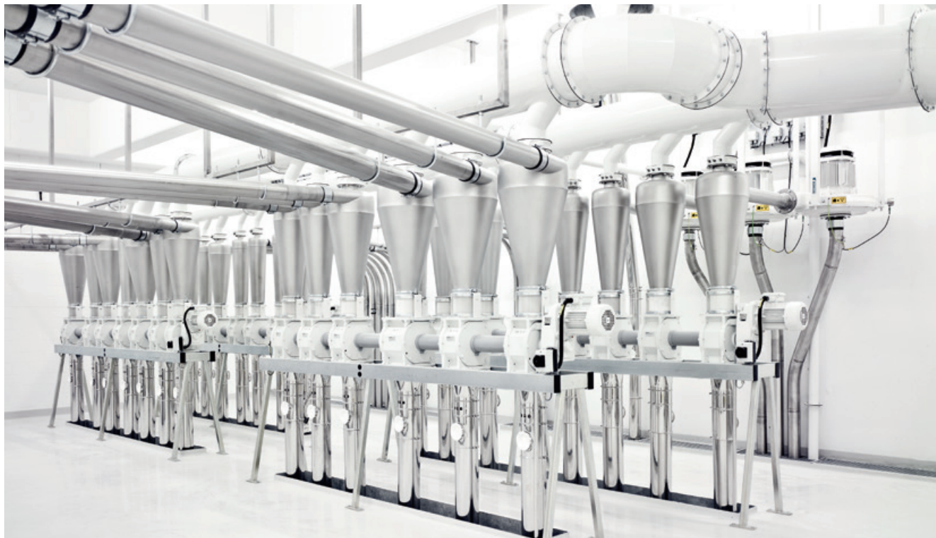
Cyclone separator MGXE. Optimal separating efficiency with high air-to-solids ratios.
