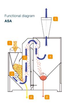
The cost-effective ASA uses exhaust air and is employed primarily for moist and / or sticky products like malt or rapeseed.
