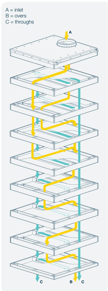
The number of sieves, the flow diagram, the stroke, and the number of fractions can be varied. Depending on the specific application and product volume, 4 to 10 sieves with 2 to 6 fractions are possible.
