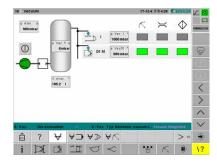
The SmartVac vacuum system is integrated seamlessly into the die-casting system. It is controlled centrally with the Ecoline S control unit. All relevant vacuum parameters are measured, monitored and assigned to the process directly – for comprehensive process transparency and optimum quality of the components.
